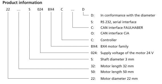
The drives integrate a brushless DC servomotor, a high-resolution encoder and a programmable position and speed controller, based on a high performance digital signal processor (DSP), within a complete drive unit.
