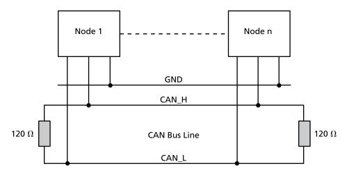
CAN is a bus system, to which all nodes are connected in parallel. A terminal resistance of 120 V must be connected to each end of the bus line.
