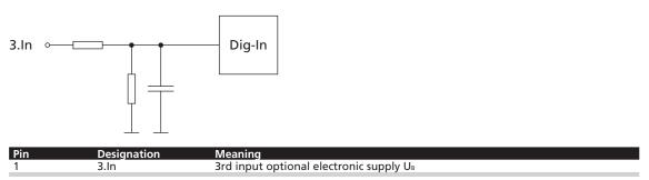
This connection can be used as reference or digital input. As an option, this input can be modified by the manufacturer to serve as a separate connection for the supply voltage to the electronics allowing the motor to be disabled independently of the electronics.
