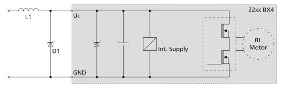
To protect against conductive emissions, we recommend plugging in the supply cable near the drive with two windings via a ferrite sleeve L1 (e.g. WE 742 700 790).
